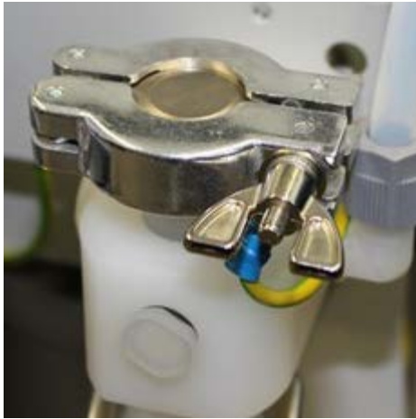
Connection with clamping ring and blind cap (delivery condition)
