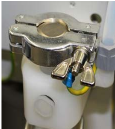
Connection with clamping ring and blind cap (delivery condition)
